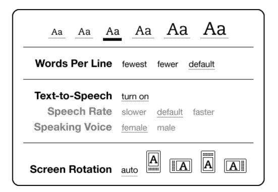
**Text key** — adjusts font size and number of words per line to suit your reading preference. Also allows you to turn on/off Text-to-Speech and to change the screen rotation settings.
